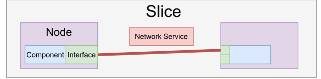
Figure 1: Main elements in a FABRIC experiment.
